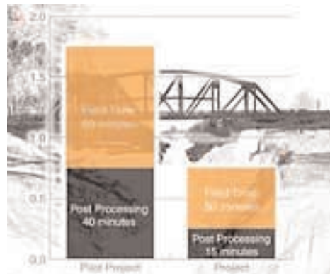
By adding more field personnel and setting up software macros to make post processing more efficient, LRA learned the benefits of scanning throughout the bridge project.
