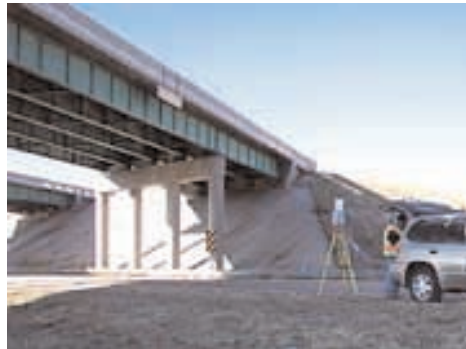
The field technician can operate the scanner from the back of his vehicle.
