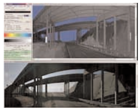
The scanning software allows the operator to obtain a photogrammetric view of the data collected on the project site right in the field on the laptop.
